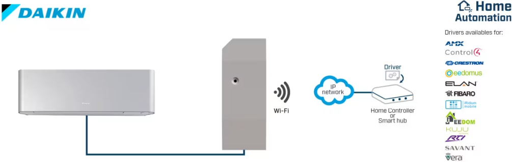
Integration of Daikin SKYAIR & VRV Systems into a Home Automation installation.
