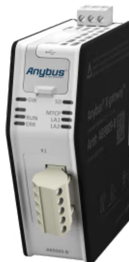
A protocol converter that connects Modbus TCP devices to CC-Link PLCs
