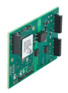
PC interface adapter (2x CAN FD), galv. isolated
