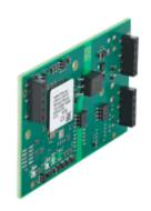
PC interface adapter (1x CAN FD), galv. isolated
