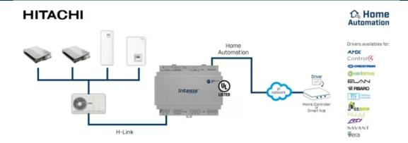
Integration example: when using the gateway to integrate mixed unit types like VRF and Ait-to-water systems.
