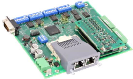
*Safe communication through Functional Safety over EtherCAT (FSoE)*
