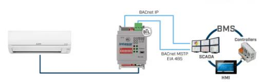
\*BACnet IP or BACnet MSTP communication selectable from switch configuration.
