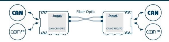
Fiber optic CAN FD repeaters enable the bridging of interference-intensive routes using optical lines. They enable complete galvanic decoupling of segments and offer high protection against overvoltage.
