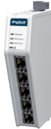
*An industrial gateway that connects Modbus TCP devices and control systems*
