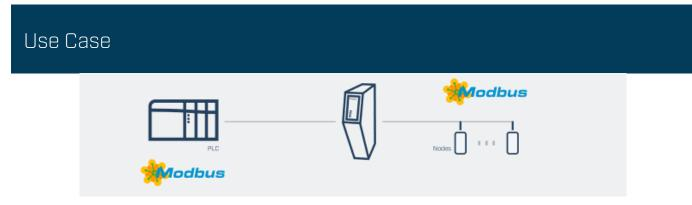
The Anybus Communicator Modbus TCP Client – Modbus TCP Server connects Modbus TCP control systems to Modbus TCP devices.
