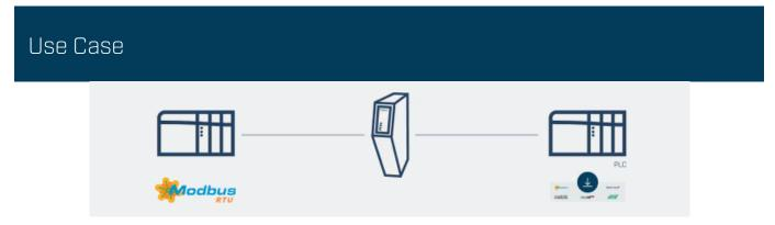
The Anybus Communicator Modbus RTU Server to Common Ethernet enables you to connect any Modbus RTU control system to any industrial Ethernet control system.
