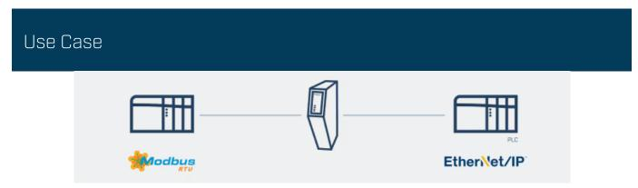
The Anybus Communicator Modbus RTU Server to EtherNet /IP Adapter enables you to connect any Modbus RTU control system to any EtherNet/IP control system.
