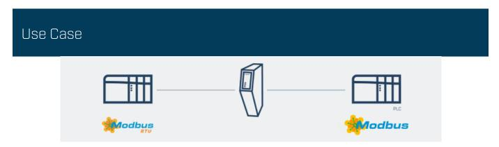
The Anybus Communicator Modbus RTU Server to Modbus TCP Server enables you to connect any Modbus RTU control system to any Modbus TCP control system.
