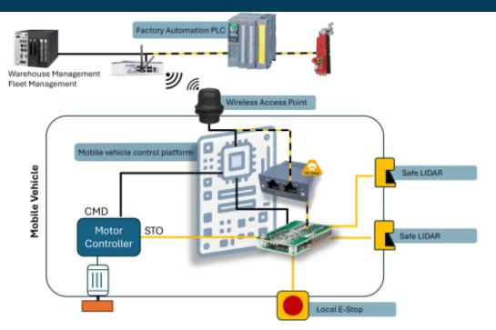
The Safe2Link Pure IO/CS enables easy integration of external safe communication into a vehicle's local safety control system. It allows local safety sensors or logic signals to be combined and routed as a single Safe Torque Off (STO) signal to the motor controller—eliminating the need for separate in-vehicle safety logic when using the SafeBound<sup>™</sup> feature.
