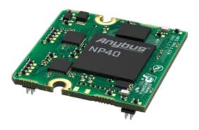
Enable communication between industrial devices and CC-Link IE TSN networks
