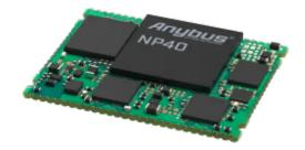
Enable communication between industrial devices and BACnet/IP networks
