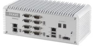
Configurable automotive platform (2 x Automotive Ethernet, 1 x FlexRay, 8 x CAN/CAN FD, 2 x LIN, and more)
