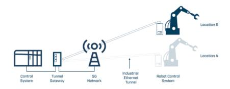
Our solution enables factories to reorganize layouts and relocate machines without the hassle of installing new cables.
