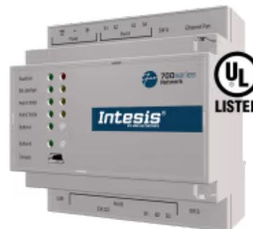
KNX zu Modbus TCP & RTU
