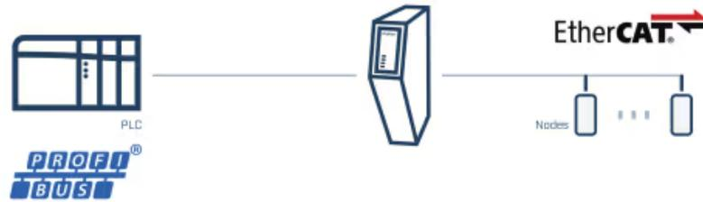
The communicator can be used wherever there is a need to transfer data between control systems using different industrial protocols.
