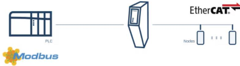
The communicator can be used wherever there is a need to transfer data between control systems using different industrial protocols.
