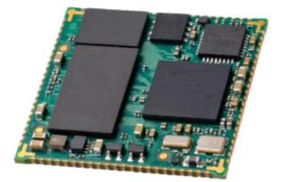
Embedded SoC controller for industrial control applications and IoT communication
