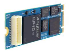
Connects computers and embedded systems to PROFINET IRT networks
