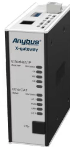
*A protocol converter that connects EtherNet/IP devices to EtherCAT PLCs*
