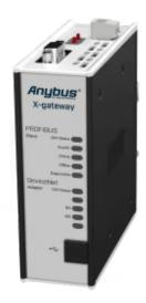
A protocol converter that connects DeviceNet and PROFIBUS control systems
