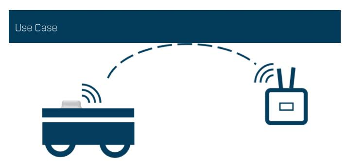
The Anybus Wireless Bolt II can be attached to roaming machines such as AGVs, enabling the machine to connect to various access points throughout the facility. It exchanges information on the best path to ensure the machine reaches its destination efficiently and safely.
