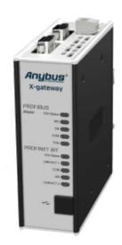
A protocol converter that connects PROFIBUS devices to PROFINET-IRT PLCs
