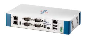
Configurable automotive platform (8x CAN, thereof 4x CAN FD)
