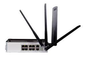
Enables a robust cellular 5G connection in an industrial production environment
