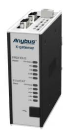
A protocol converter that connects PROFIBUS devices to EtherCAT PLCs
