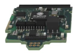
Enable communication between industrial devices and PROFINET IO 2-Port networks
