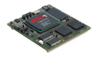
An Computer on Module built on the highly integrated 32-bit Power Architecture  $^{\text{IM}}$  technology. Designed for demanding control and intensive network communication tasks.
