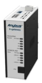
A protocol converter that connects DeviceNet devices to POWERLINK PLCs
