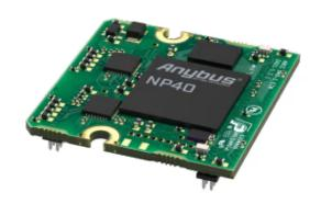
Enable communication between industrial devices and BACnet/IP networks
