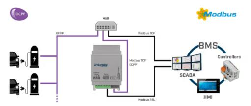
Integration of OCPP EV Charging points into a Modbus installation.
