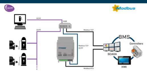
Gateway acting as an OCPP bridge between an OCPP Central System and OCPP chargers.
