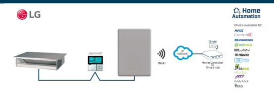
Integration of LG Commercial line and VRF Air Conditioners Units into a Home Automation installation.
