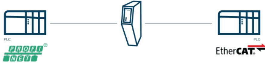
The communicator can be used wherever there is a need to transfer data between control systems using different industrial protocols.
