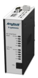
A protocol converter that connects AS-Interface devices to FIPIO PLCs
