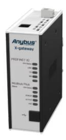
A protocol converter that connects Modbus Plus and PROFINET-IO control systems
