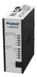
A protocol converter that connects AS-Interface devices to Interbus CU PLCs
