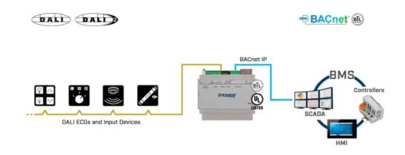
Integration of DALI drivers and sensors into a BACnet installation.
