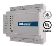
M-BUS to BACnet/IP & MS/TP - 20 devices
