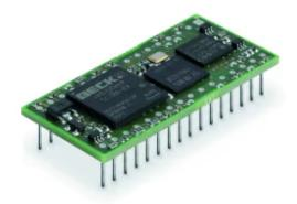
An embedded SoC web controller with a DIL32 footprint for for Smart Grid Applications
