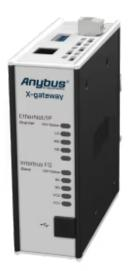
A protocol converter that connects EtherNet/IP devices to Interbus FO PLCs
