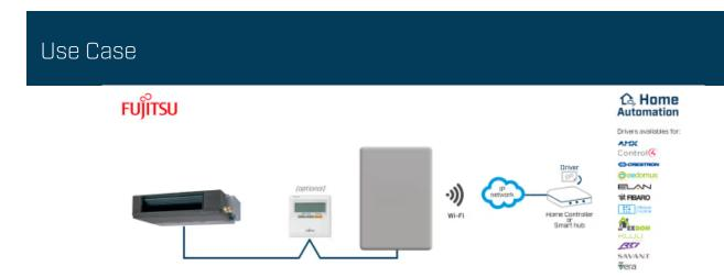
$Integration \ of \ Fujitsu \ Air \ Conditioner \ Systems \ into \ a \ Home \ Automation \ installation.$
