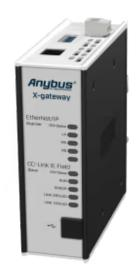
A protocol converter that connects EtherNet/IP devices to CC-Link IE Field PLCs
