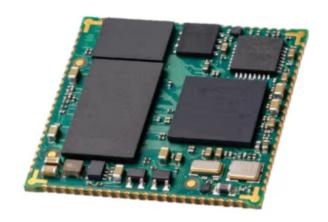
Embedded SoC controller for IEC 61131-3 runtime system
