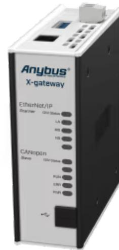
*A protocol converter that connects EtherNet/IP devices to CANopen PLCs*
