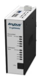
A protocol converter that connects DeviceNet devices to CANopen Slave PLCs
