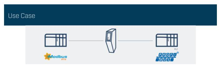
The Anybus Communicator Modbus RTU Server to PROFIBUS IO-device enables you to connect any Modbus RTU control system to any PROFBUS IO control system.
